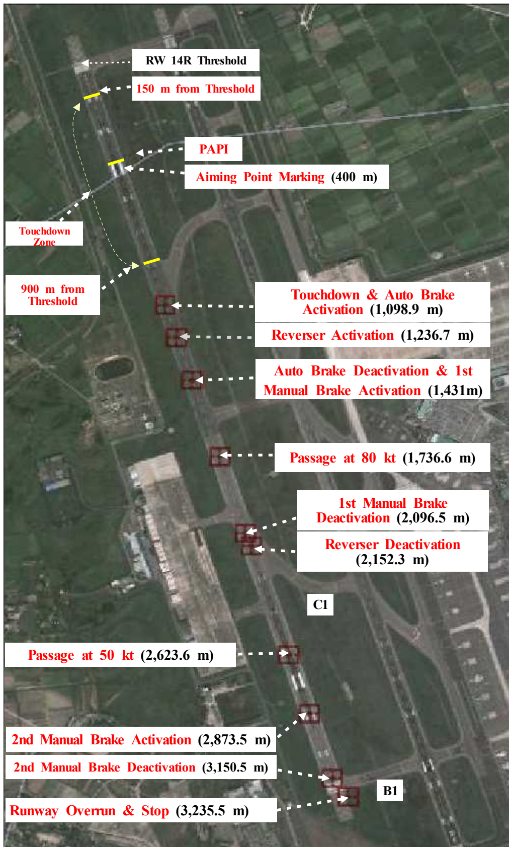
[Figure 11] Positions of the Braking System Operation During Landing
