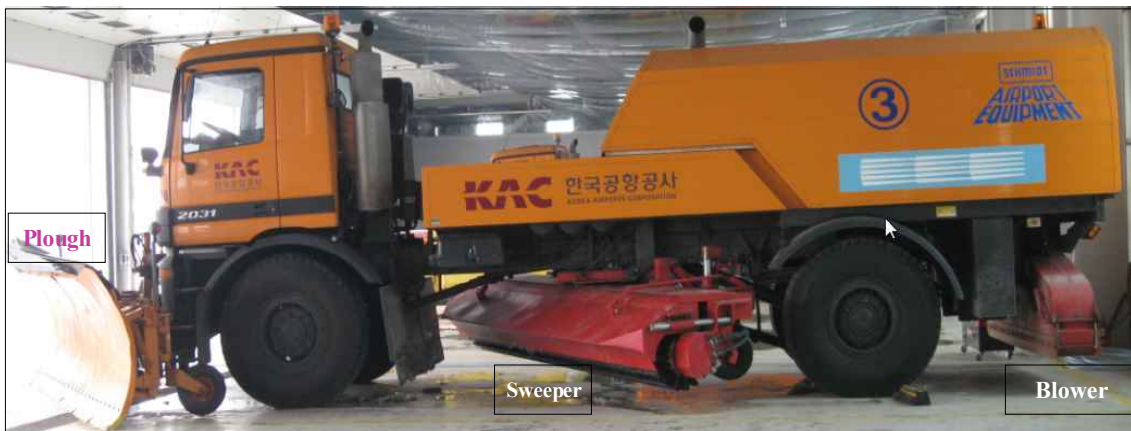
[Figure 6] Multipurpose (Plough, Sweeper, Blower) Snow Removal Truck
