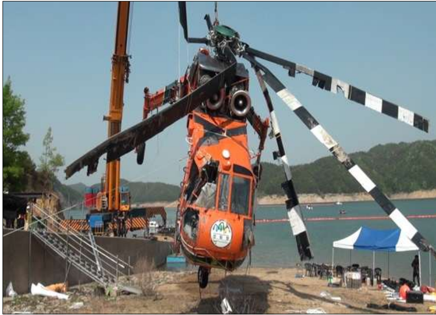
[Figure 13] Damage to Main Rotor Blades (during recovery)
