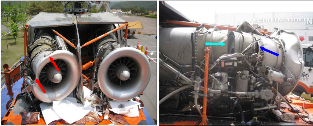
[Figure 14] External Damage of RH Engine
