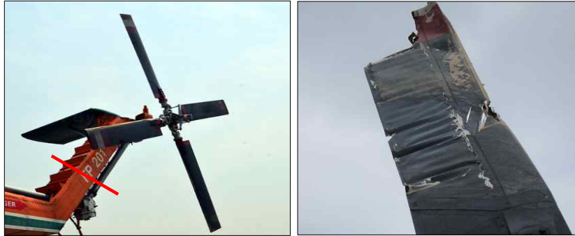
[Figure 20] Aft Severed Portion of the Tail Boom and Tail Rotor Damage
