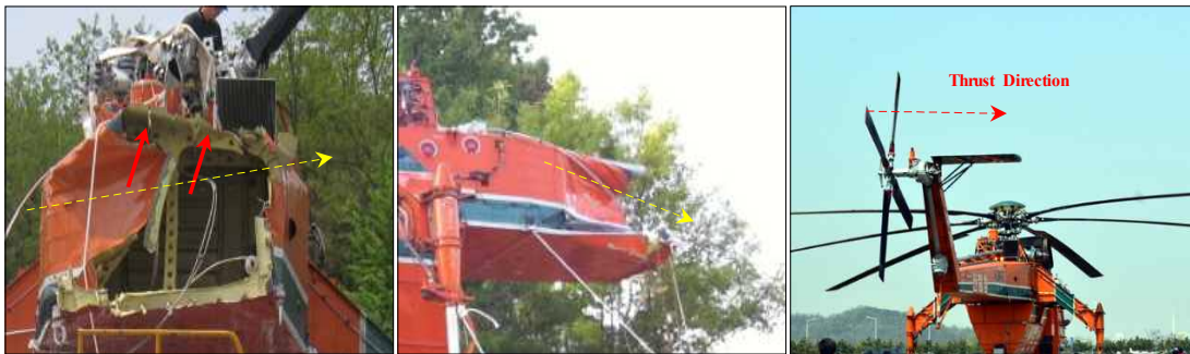
[Figure 19] Forward Severed Portion of the Tail Boom and the Tail Rotor's Thrust Direction
