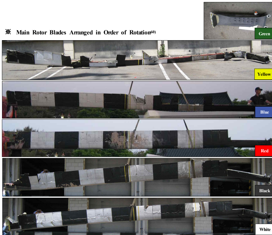
[Figure 13-1] Damage to Main Rotor Blades (upper side)
