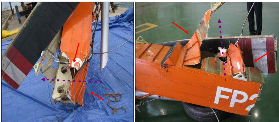
[Figure 11] Fracture Surface of the Aft Portion of the Tail Boom (red arrow) and Fracture Direction (purple arrow)
