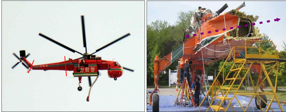
[Figure 10] Tail Boom Fractures and Fracture Surface of the Forward Portion
