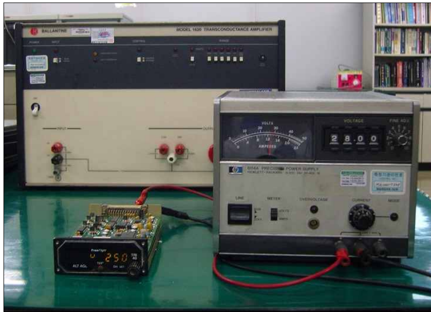
[Figure 9] Decision Height Set in the Radio-Altimeter
