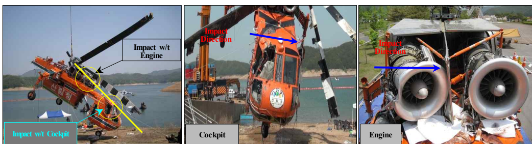
[Figure 21] Damage to RH Engine and Upper Portion of Right Pilot Seat
