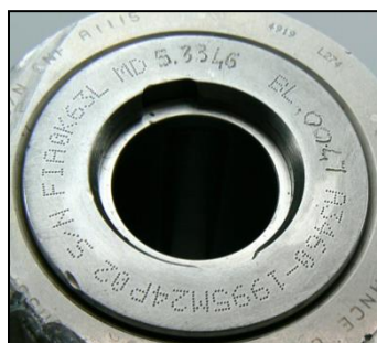
PHOTO 3: RADIAL GEARSHAFT MARKINGS (INNER DIAMETER – OUTER DIAMETER IS BEARING RACE)
