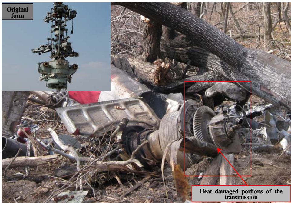
[Photo 6] Damaged portions of the transmission and mast
