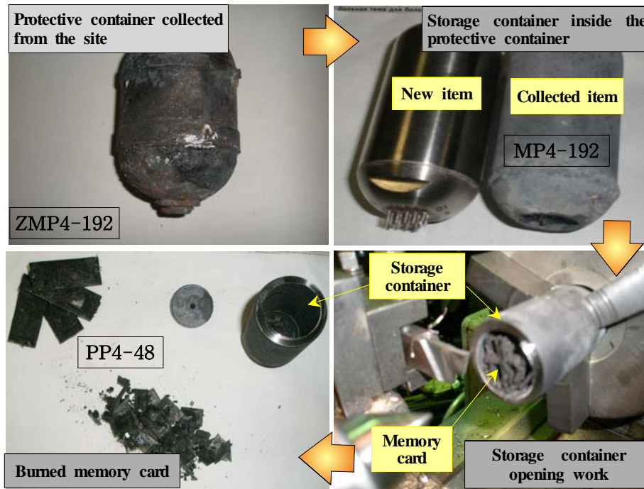
[Photo 4] Protective container collected from the site and the oxidized memory card
