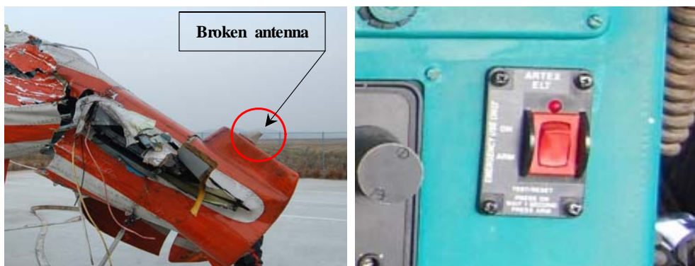
[Photo 8] Damage to ELT antenna and switch condition
