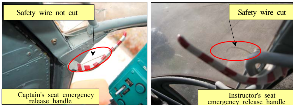
[Photo 9] Exit door emergency release handle safety wire condition
