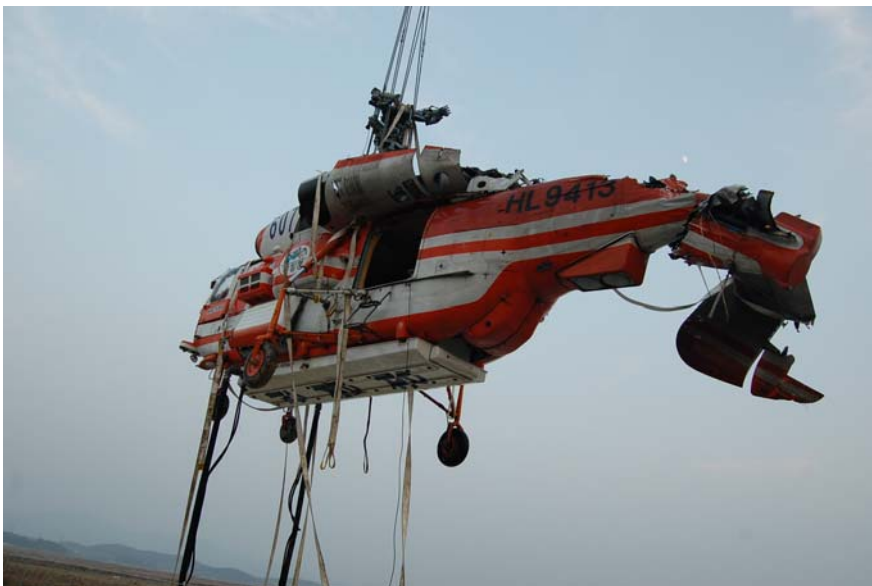
[Photo 2] HL9413 under salvage work
