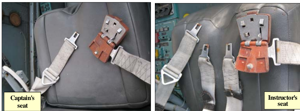
[Photo 11] Cockpit seat belts of captain's seat and instructor's seat
