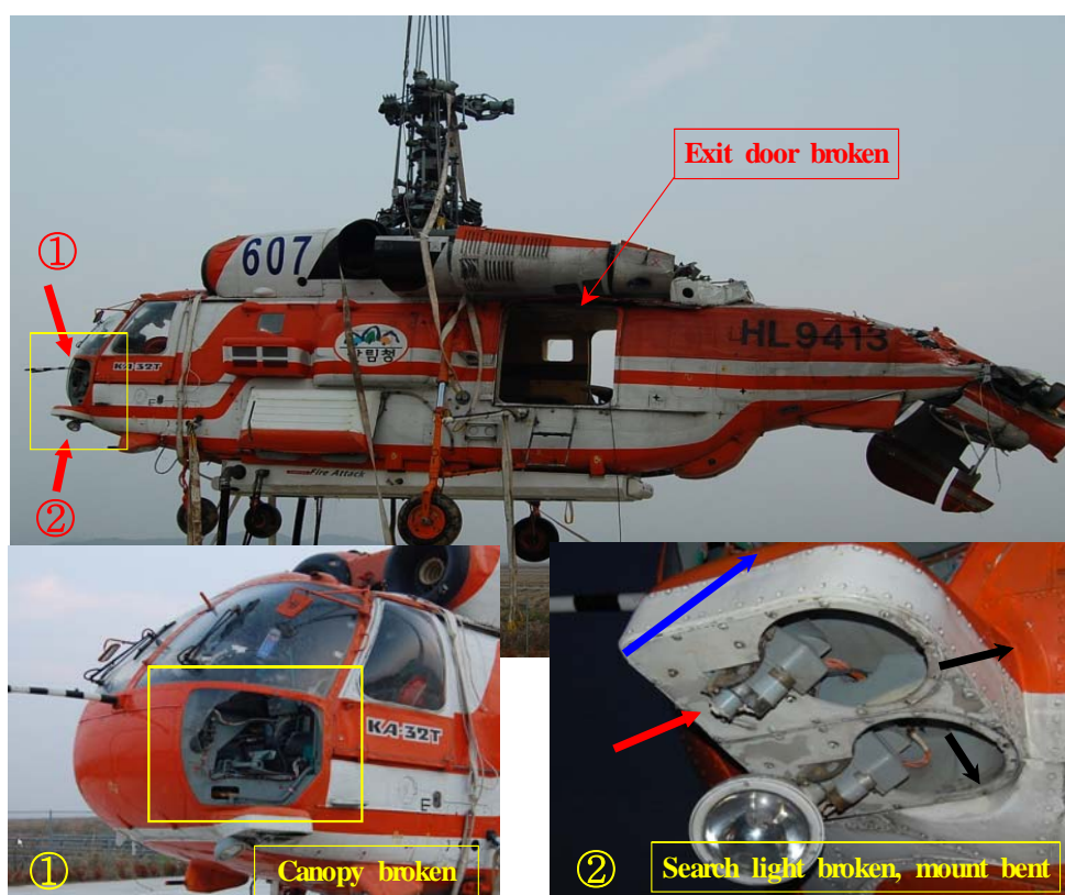
[Photo 3] Main damaged portions of fuselage
