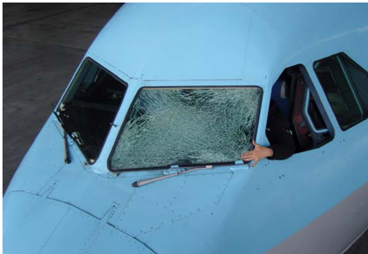
[Photo 1] L1 windshield damaged
