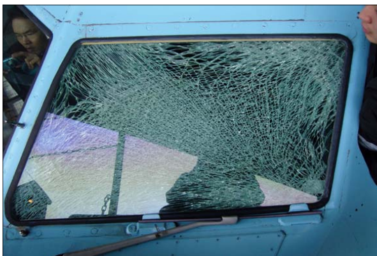
[Photo 2] Damaged windshield (L1)
