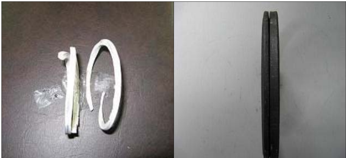
[Photo 2] Damaged Seal(Left)
