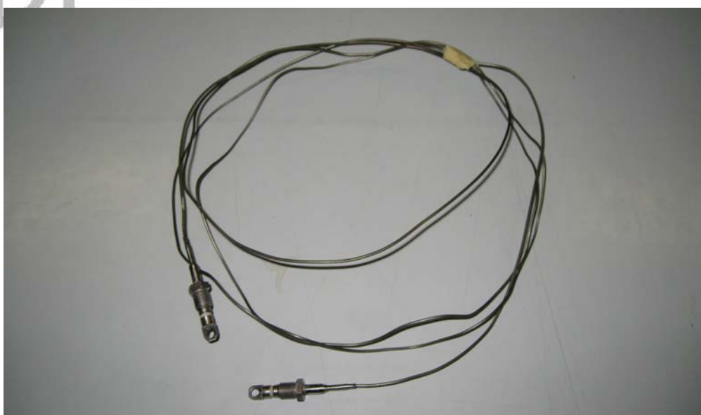
[Figure 2] JET/PIPE Sensing Element Removed
