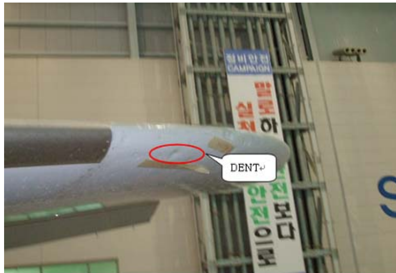
[Photo 4] Damage to horizontal stabilizer 1
