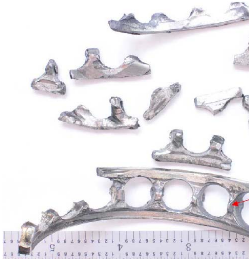
[Photo 7] Damage to ball bearing cage
