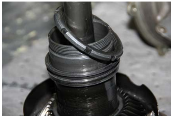
[Photo 8] Loosened AB-1 bearing inner race retaining nut
