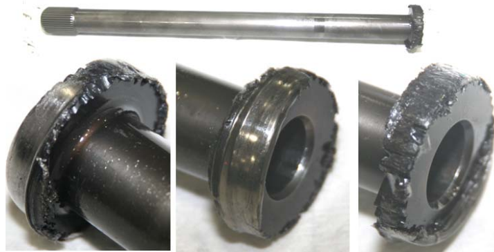
[Photo 5] Damage to towershaft splines
