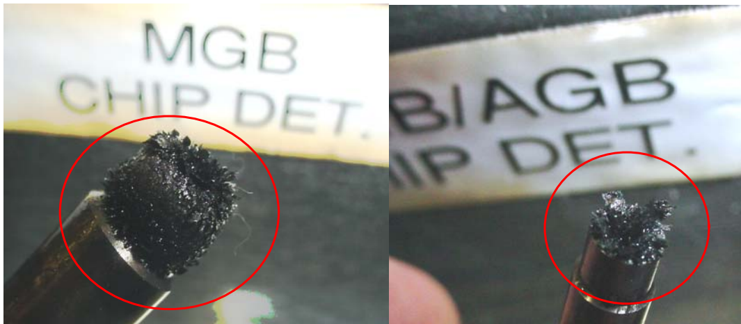
[Photo 1] Metal chip found in the main gearbox and angle gearbox.
