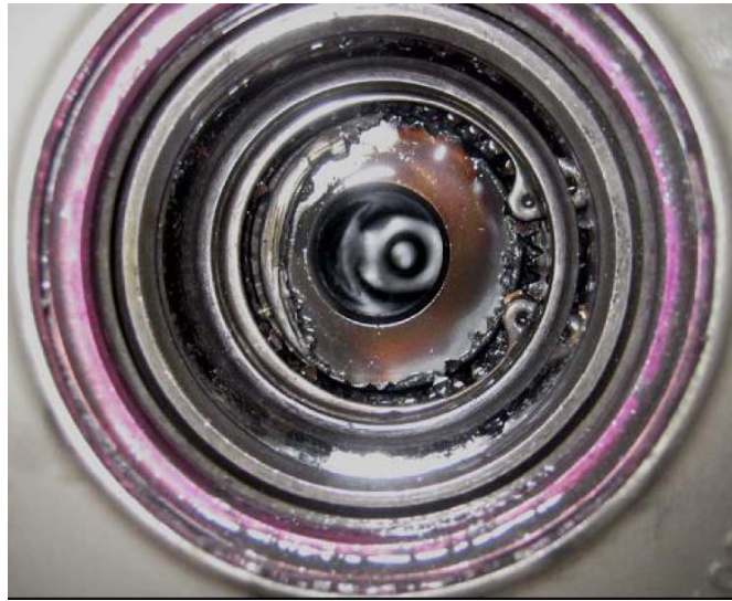
[Photo 3] Damage to towershaft bottom splines
