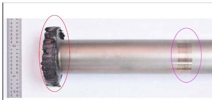
[Photo 4] Damage to towershaft
