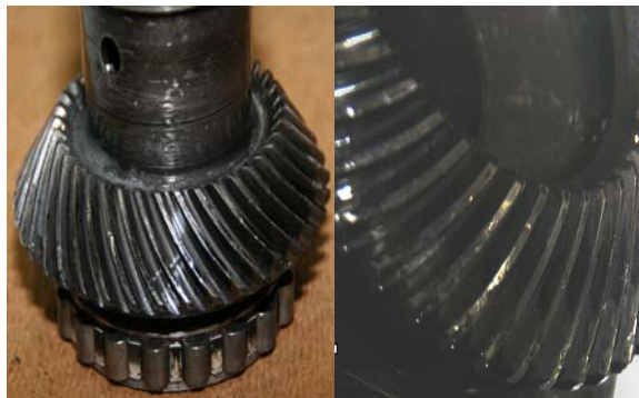
[Photo 12] Damage to bevel gear
