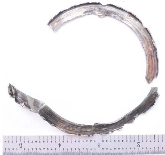
[Photo 9] Damaged retaining nut lock washer
