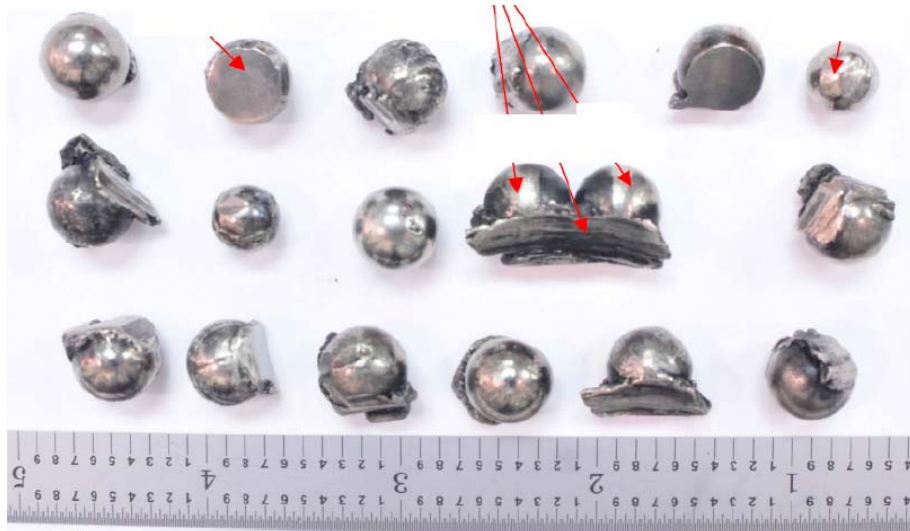
[Photo 10] Damaged bearing balls
