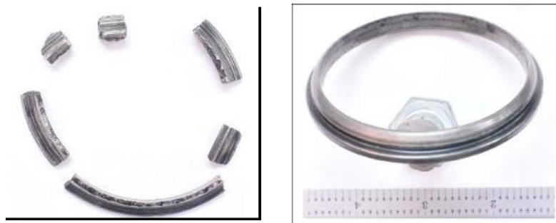
[Photo 6] Damage to AB-1 bearing inner race
