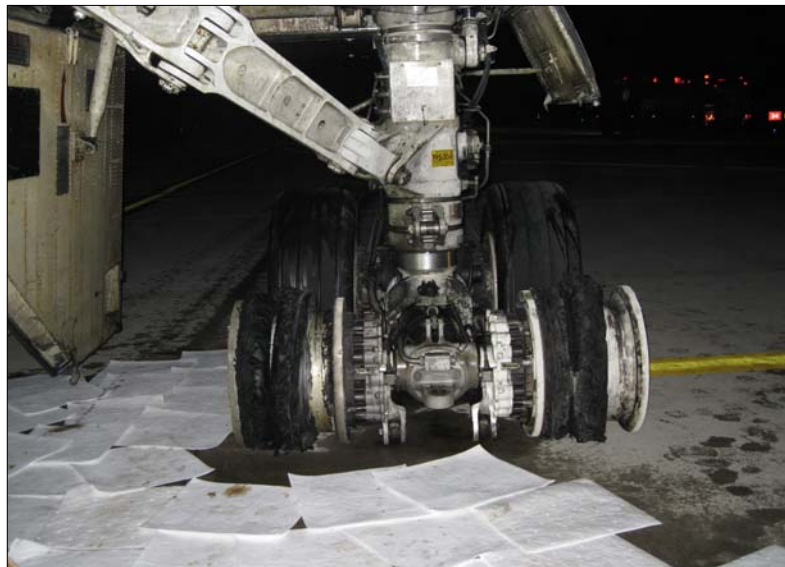
[Photo 1] Damaged number 5 and 6 tires
