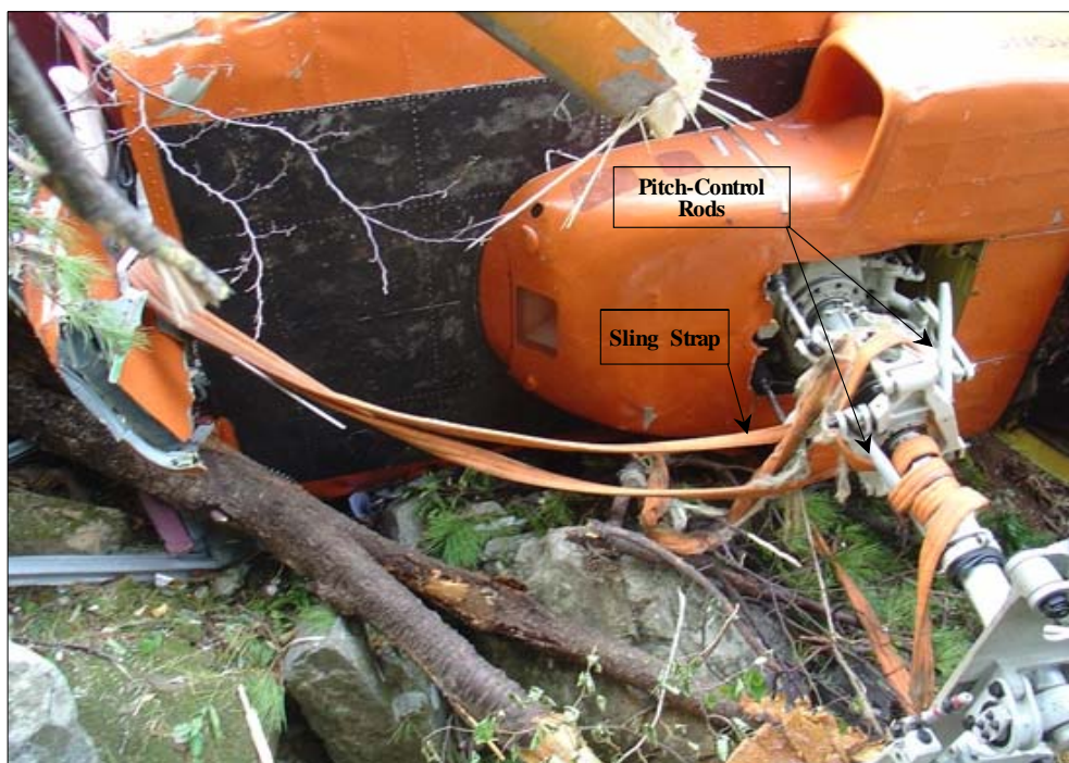
[Figure 12] Sling Strap Wrapped Around the Mast and the Fractured Pitch-control Tubes
