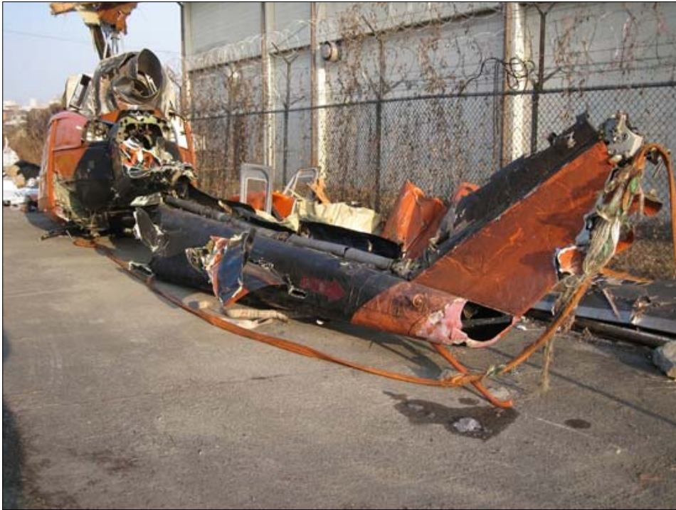
[Figure 15] Comparison of the Damaged Location of the Sling Strap with the Location of the Tail Rotor
