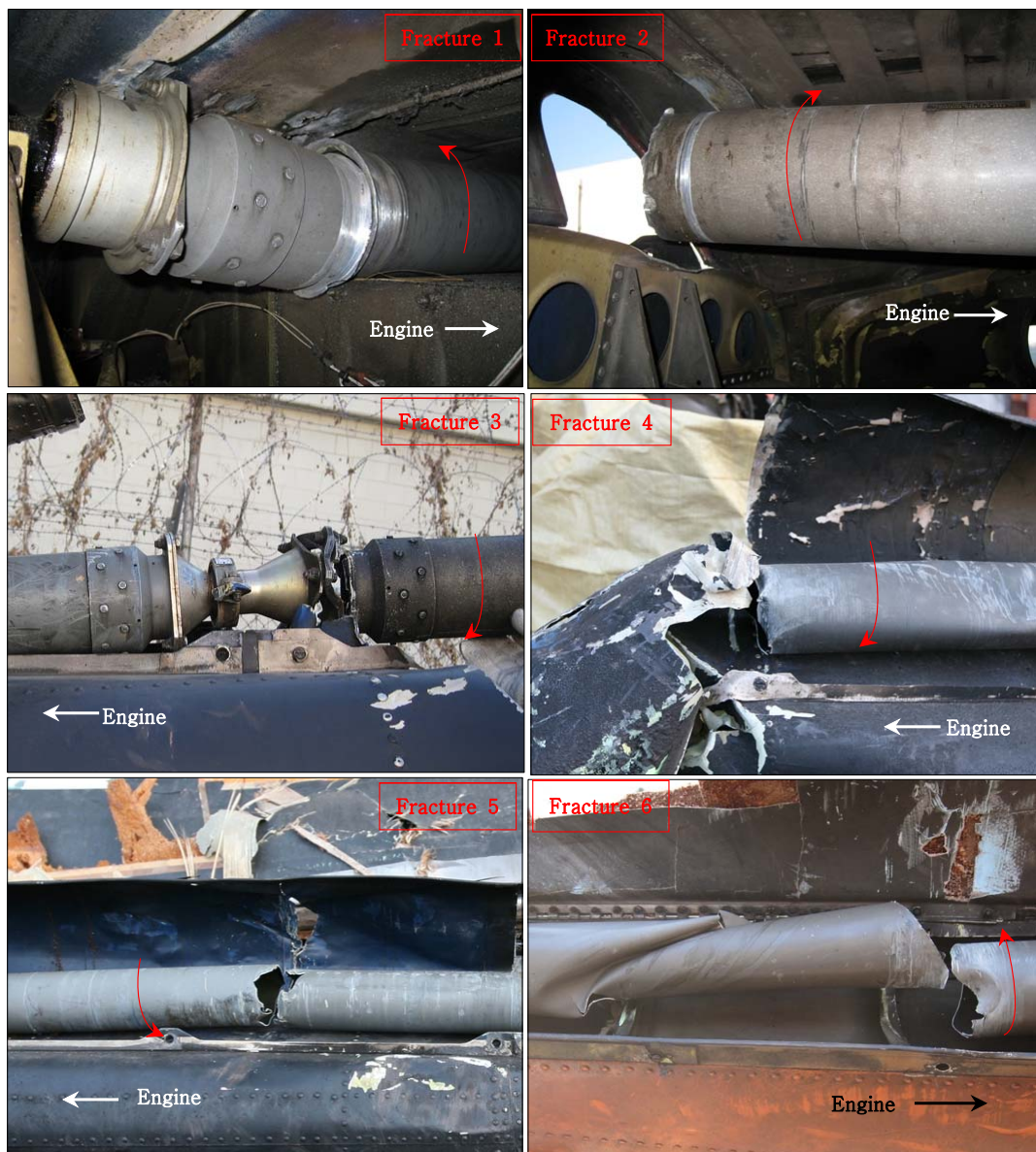
[Figure 8] Fracture Surfaces of the Tail Rotor Driveshaft
