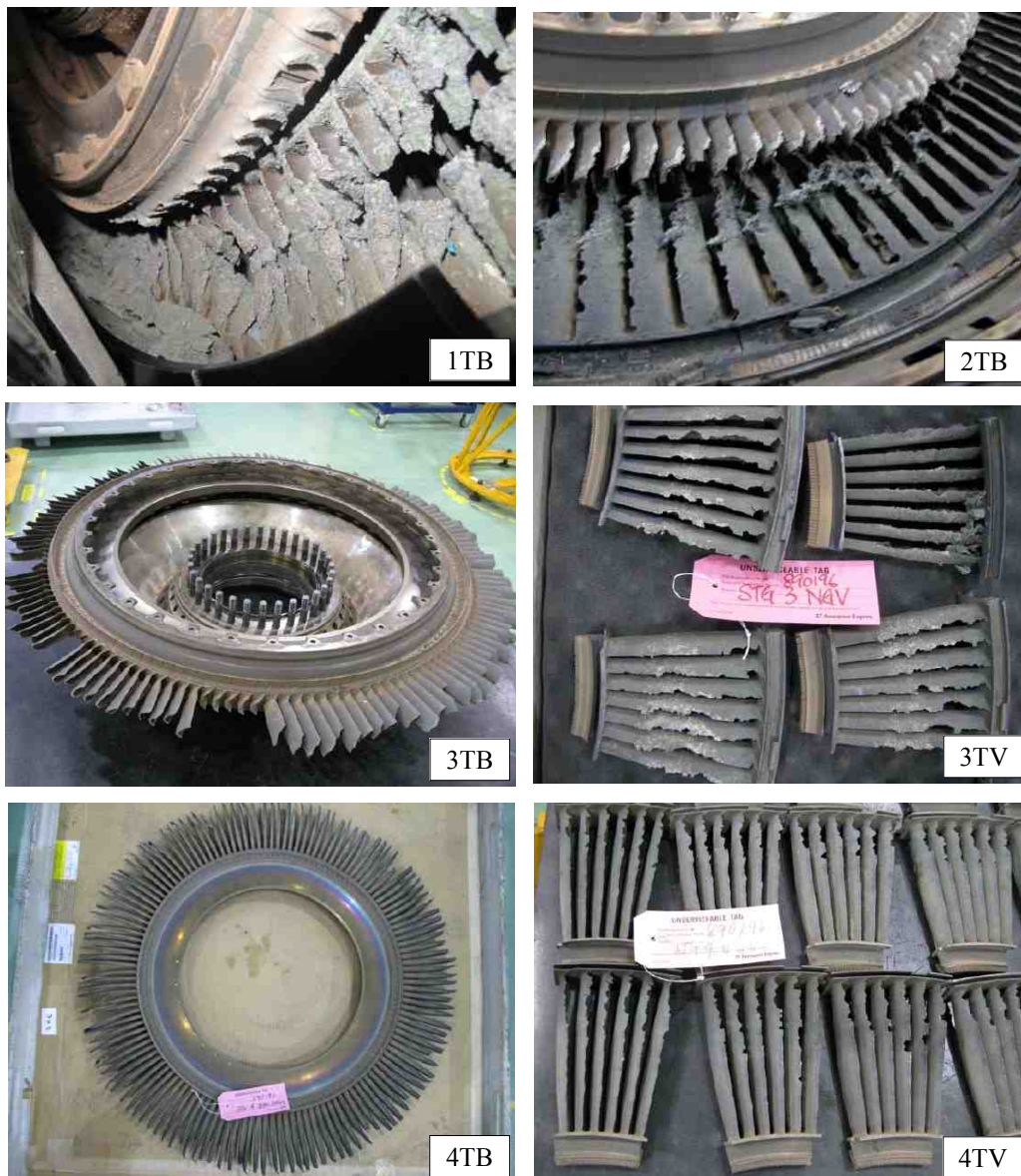
[Figure 8] Stage-by-stage Damage of the LPT Blades and Vanes
