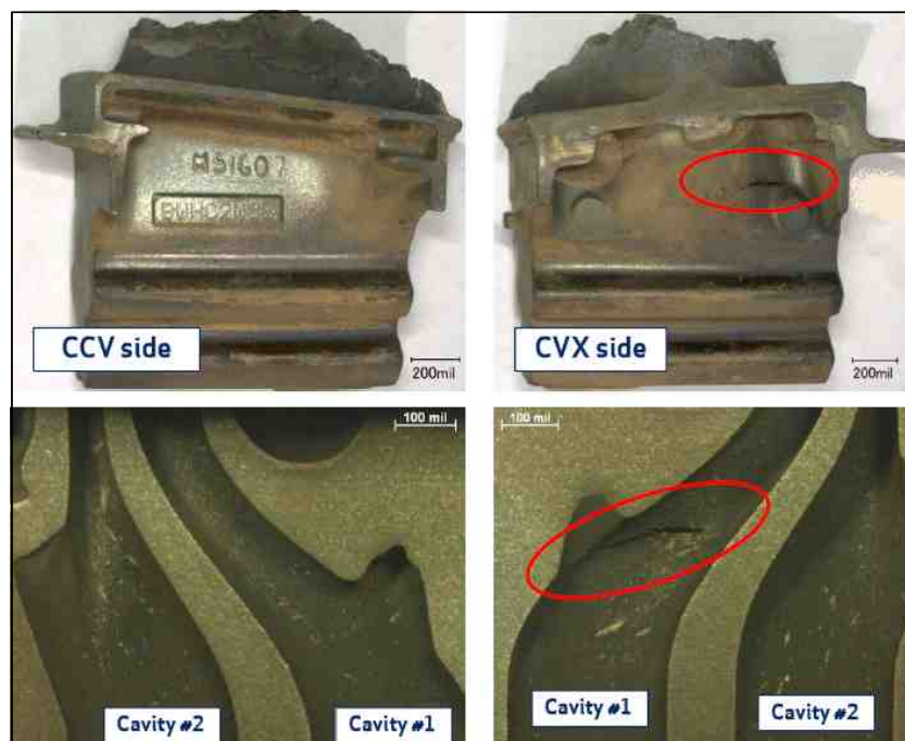
[Figure 11] Through Wall Transition Zone Crack
