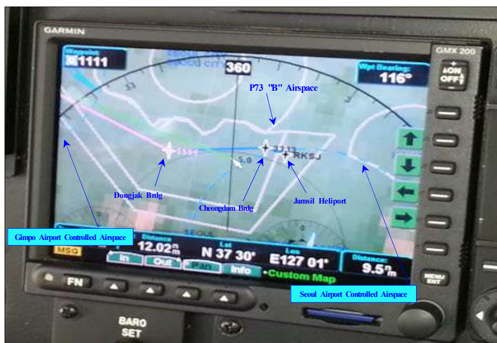
[Figure 5] Screen of the Same Model GPS on the Same Type Aircraft
