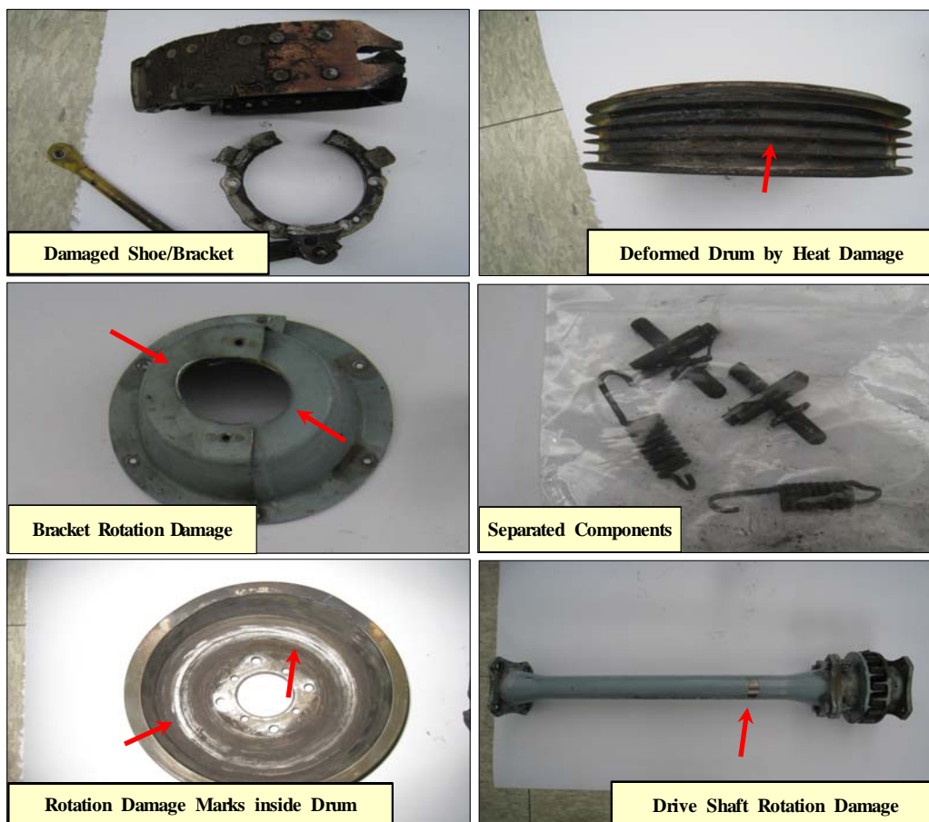
[Photo 3] Damaged Components Removed
