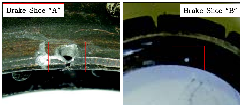
[Photo 6] Damage in Return Spring Connector of Brake Shoe
