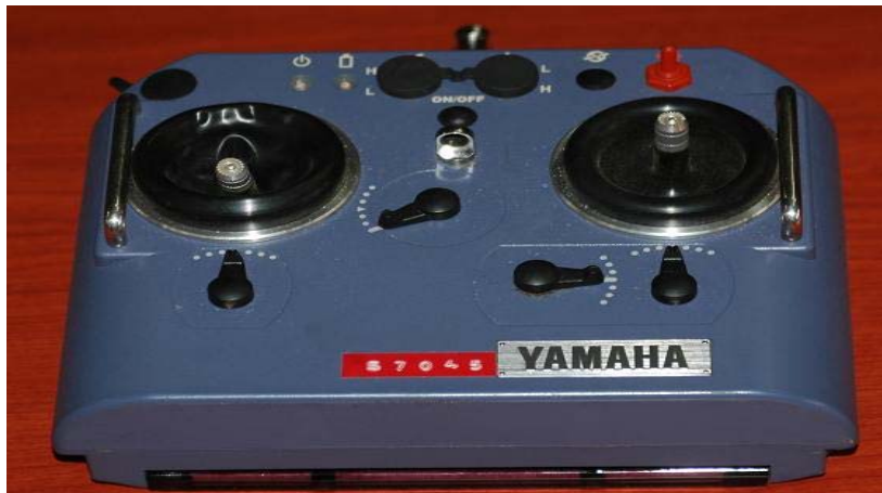
Photo 7. Various trim switches of the radio control box
