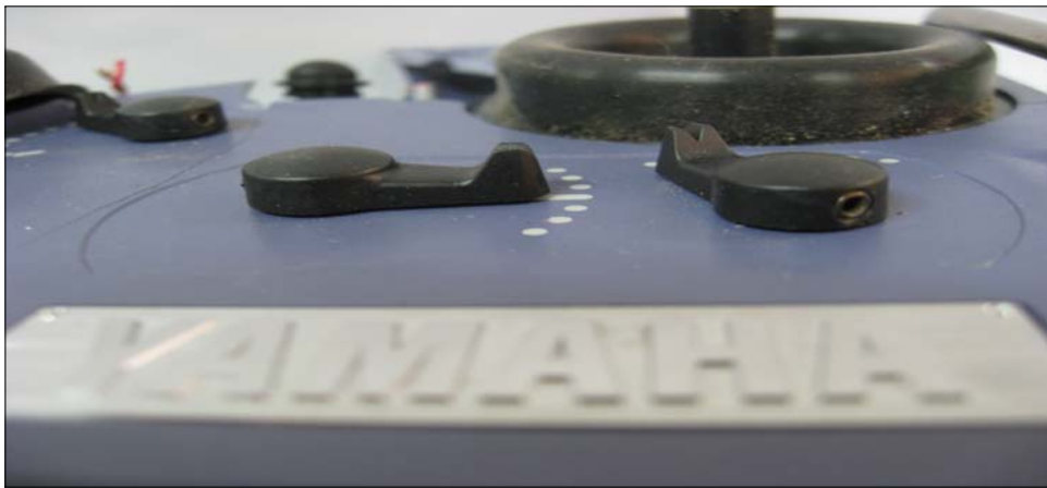
Photo 9. Convex trim switches on the panel of radio control box
