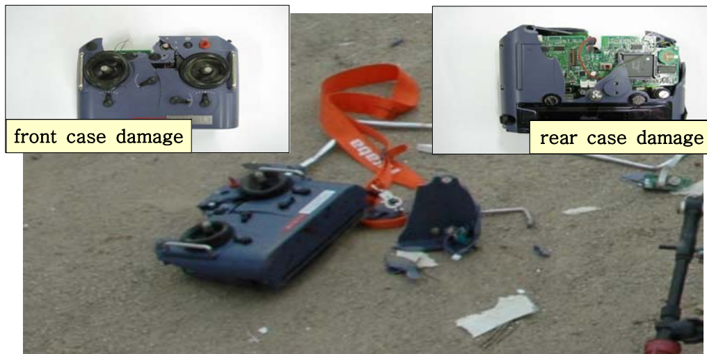
Photo 6. damaged radio control box found at the site
