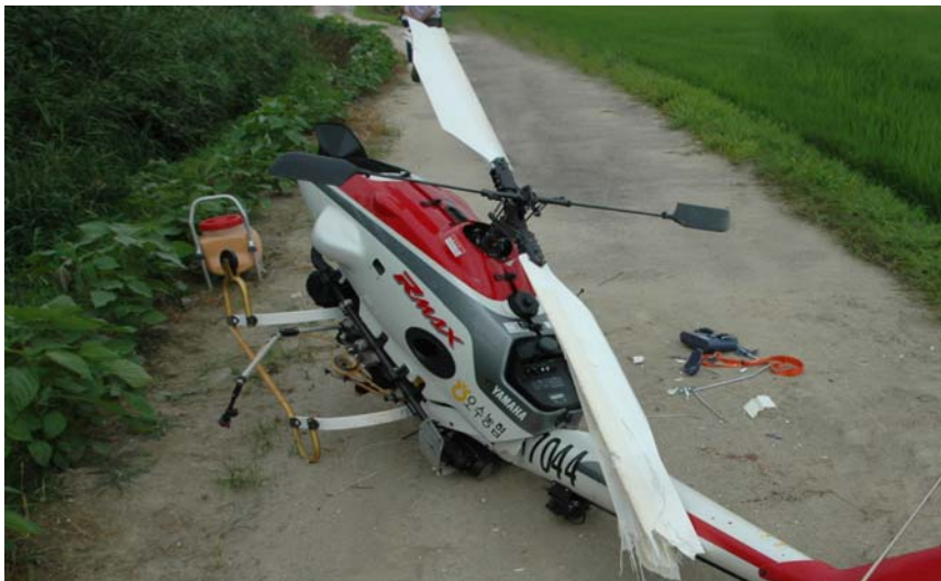
Photo 3. Main rotor damaged
