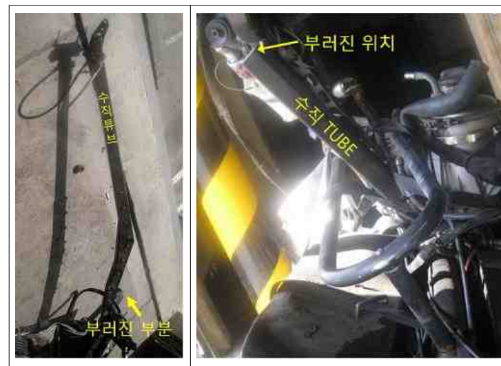
[Figure 10] Broken Vertical Tube
