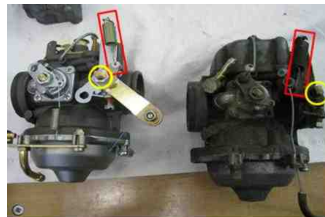
[Figure 2] Delivered Carburetor (left) &amp; Modified Carburetor (right)
