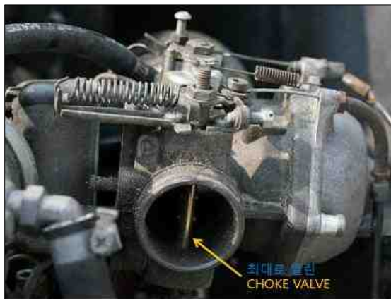
[Figure 13] Choke Valve in the Full Open Position
