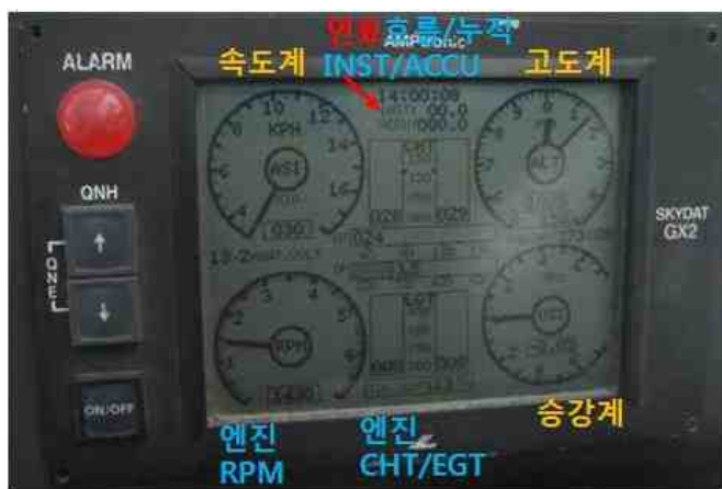
[Figure 17] S1045's SKYDAT GX2 Instrument Panel
