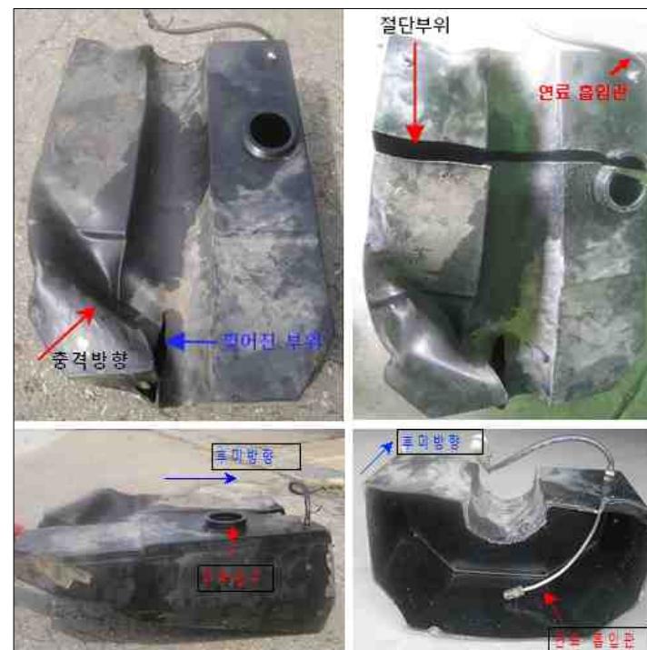
[Figure 12] Damaged Fuel Tank (left) and the Tank Cut (right)
