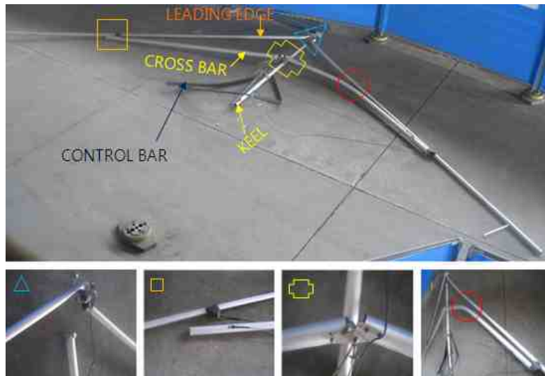
[Figure 15] Inner Structure of the Wings and its Damage
