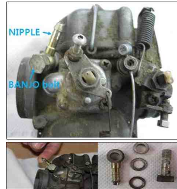
[Figure 3] Carburetor Contaminated by a Loose Banjo Bolt
