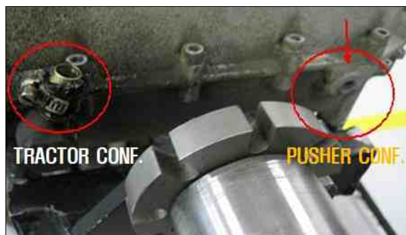
[Figure 4] Oil Return Line Installed at a different position
